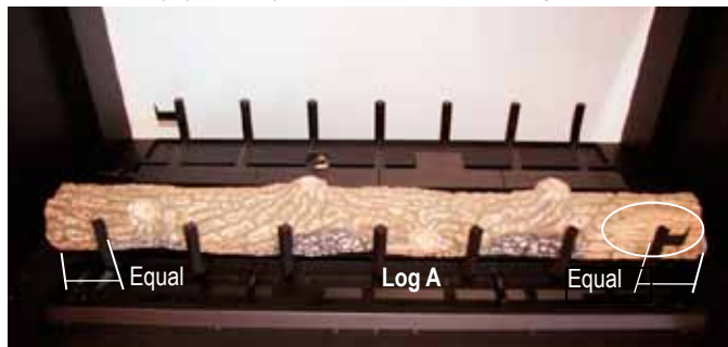
Figure. 11a Placing the First Log labelled 'A'. (Note: Location of knots and location of stripped faux bark, indicated by oval at right end). (Both 'A' logs Typical).
