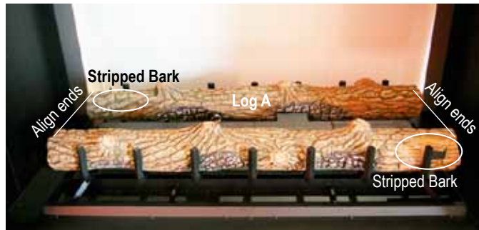
Figure. 11b Placing the Second Log labelled 'A'. (Align ends of both Logs).
