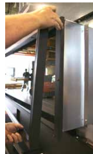
Figure 15. Step 2. (removal of Trim)
