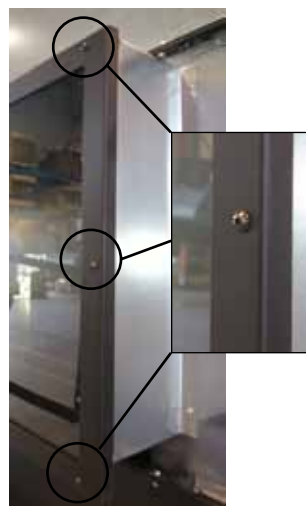
Figure 16. Step 3 (Removal of Door Frame)
