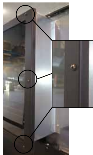
Figure 16. Step 3 (Removal of Door Frame)
